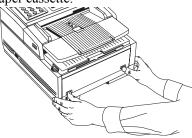
3. Pull the manual paper feeder down until it is horizontal.
